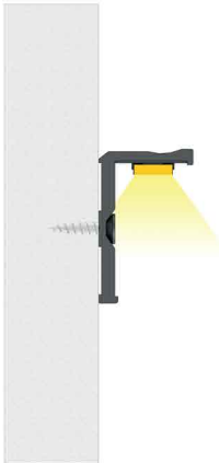
The end result of the installation of profile E using a mounting screw
