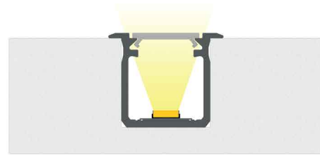
The end result of installation of groove mounted profile G with a BASIC cover
