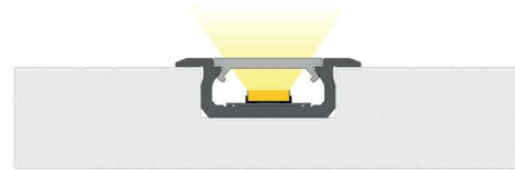
The end result of installation of groove mounted profile Z with a BASIC cover
