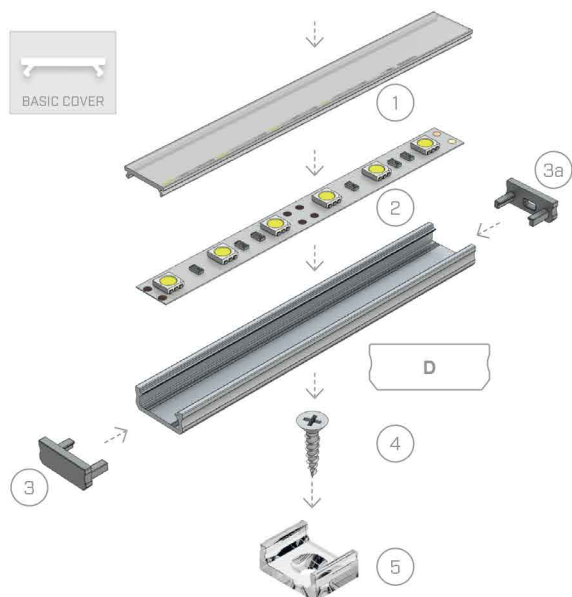
Assembly scheme for elements of the lighting system using profile D and (1) BASIC cover, (2) LED strip (3) end cap without hole, (3a) end cap with hole, (4) screw, (5) MINI mounting clip for profile D
